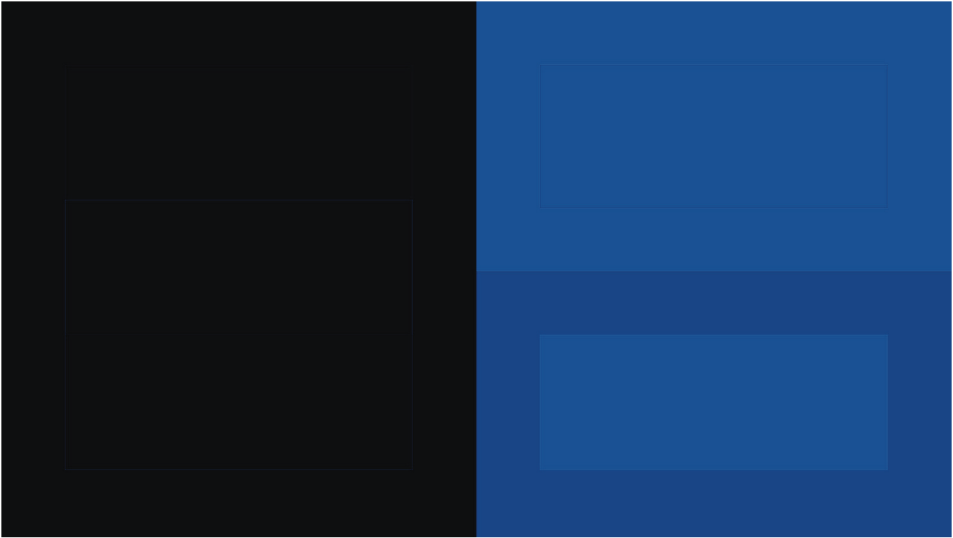
Fig. 13e: If the display's Tint setting is set too high, you will see a lighter blue rectangle in the lower part of the blue area. (Menu: SDR BT.709 | Setup)
