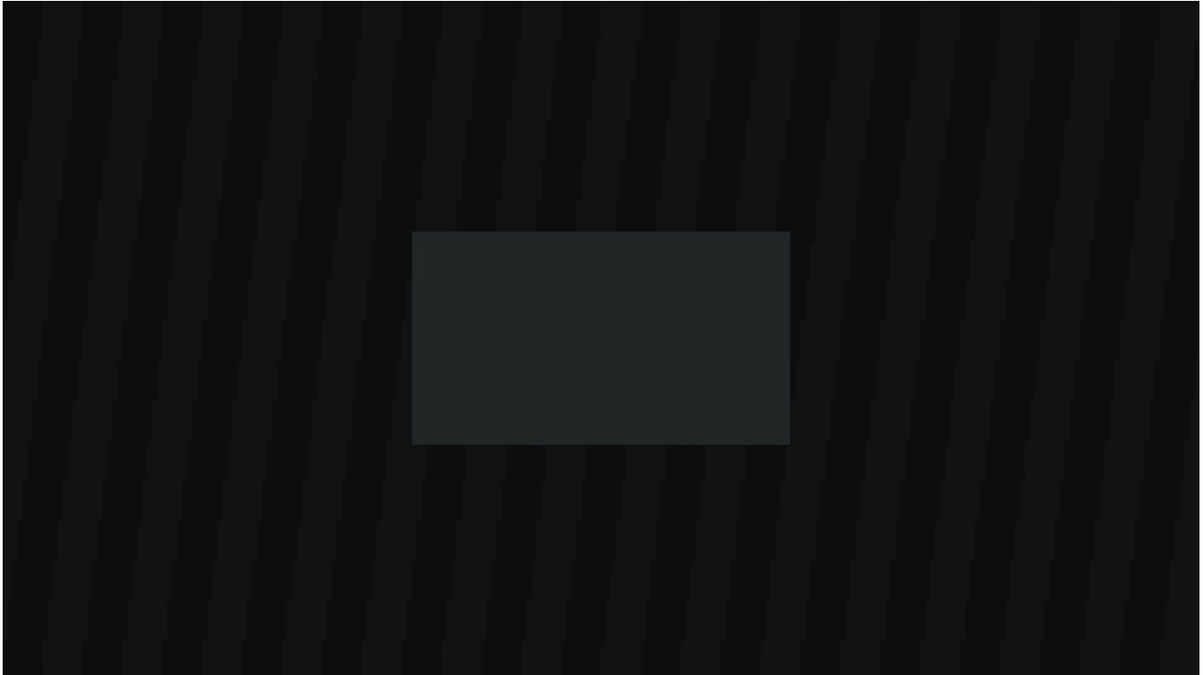
Fig. 9: Set the brightness of the bias light to roughly match the brightness of the central rectangle in the Bias Light pattern. This setting will be different for HDR and SDR. (Menu: Video Setup and SDR BT.709 | Setup)
