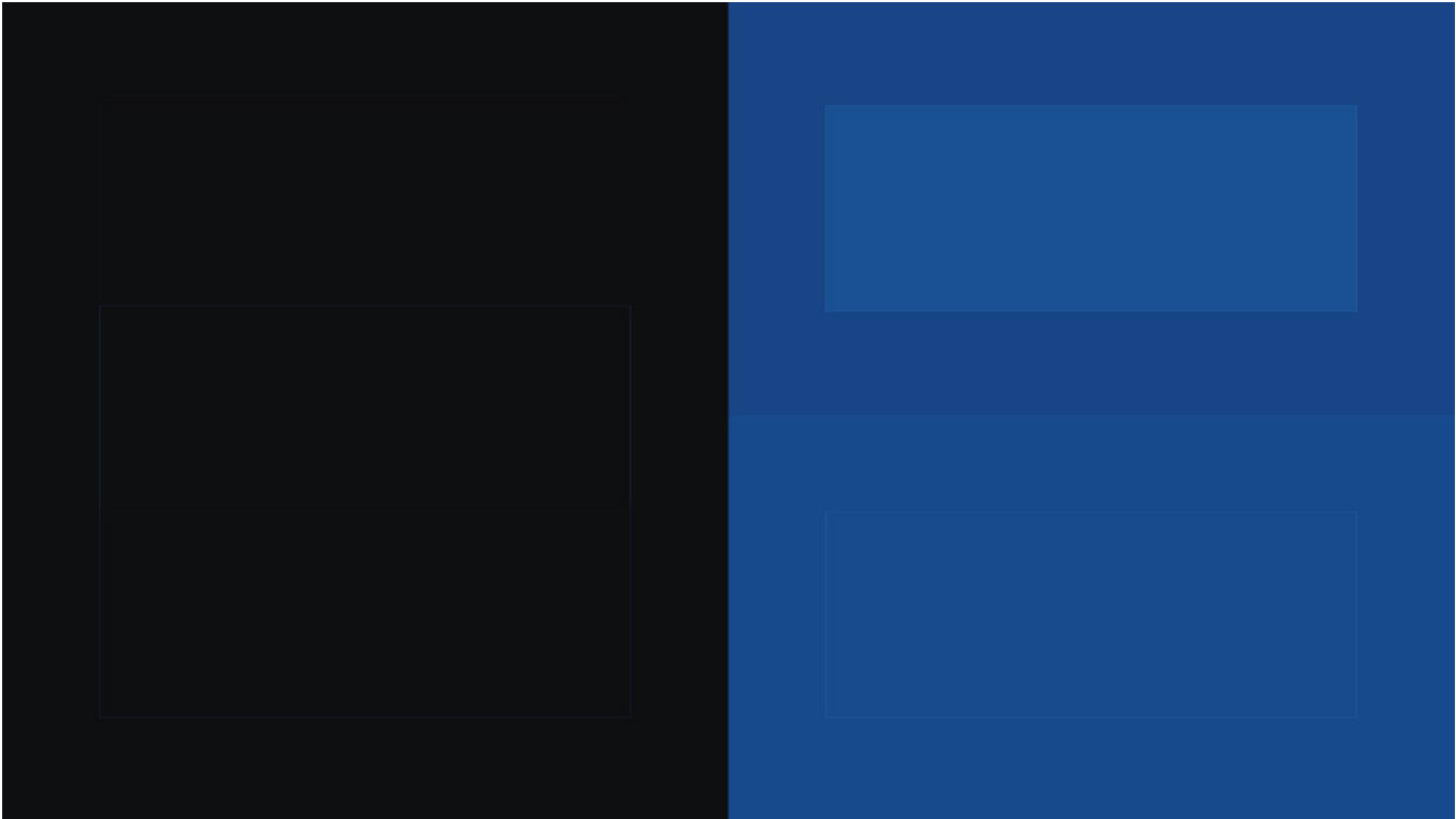
Fig. 13c: If the display's Color setting is set too high, you will see a lighter blue rectangle in the upper part of the blue area. (Menu: SDR BT.709 | Setup)
