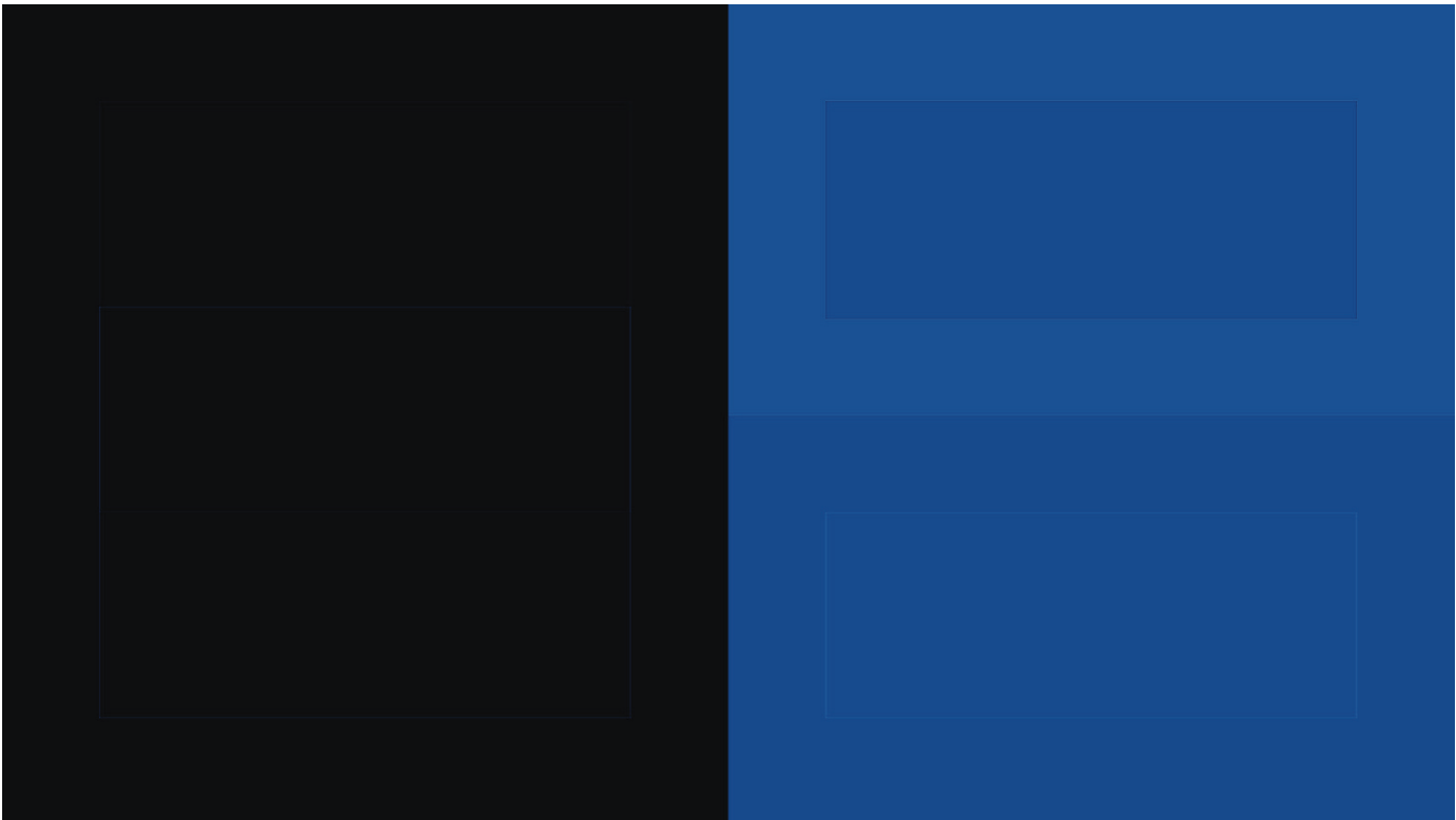
Fig. 13d: If the display's Color setting is set too low, you will see a darker blue rectangle in the upper part of the blue area. (Menu: SDR BT.709 | Setup)
