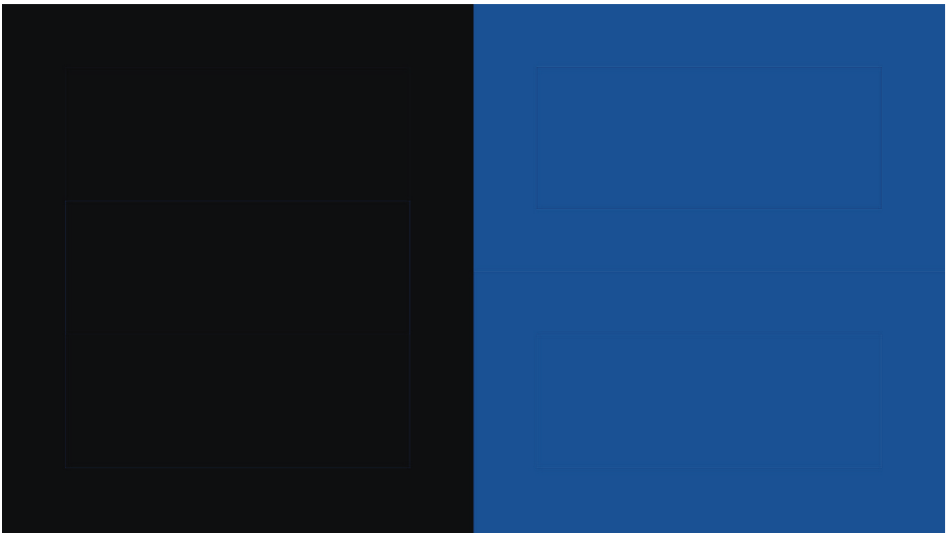
Fig. 13b: If the display's Color and Tint controls are set correctly, the Color and Tint pattern will look uniform black on the left and uniform blue on the right when viewed in the display's blue-only mode. (Menu: SDR BT.709 | Setup)
