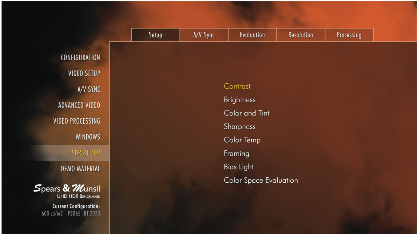
Fig. 10: To optimize your display's SDR performance, select SDR BT.709 in the main menu along the left side and Setup in the submenu along the top.
