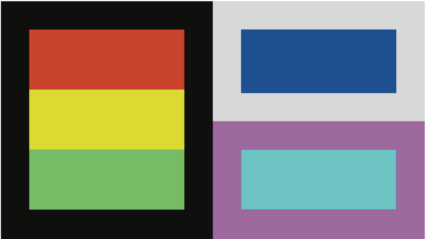
Fig. 13a: Here's the Color and Tint pattern in full color with no blue filter or blue-only mode.
