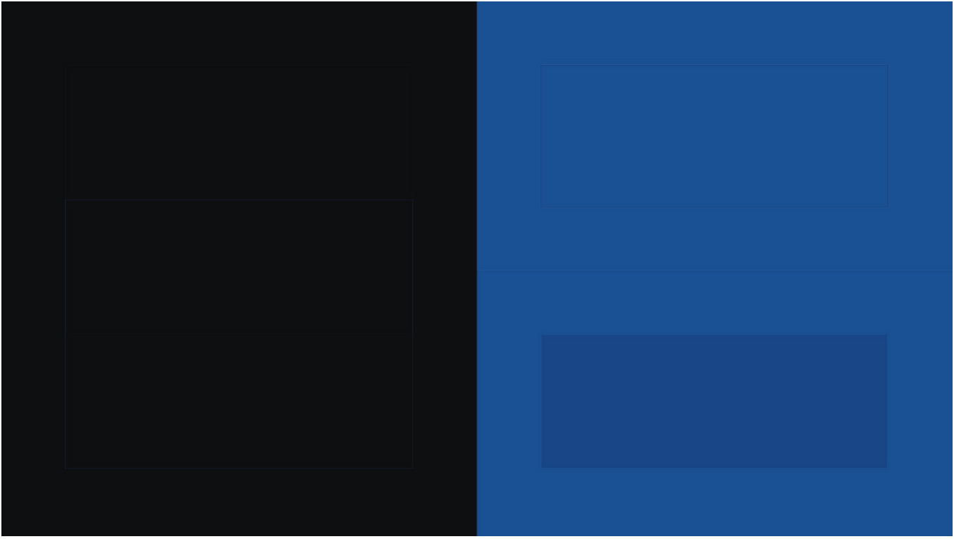
Fig. 13f: If the display's Tint setting is set too low, you will see a darker blue rectangle in the lower part of the blue area. (Menu: SDR BT.709 | Setup)
